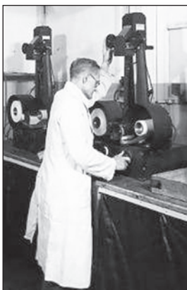
Figure 7. Airgraph enlargements being made from the spool of miniature film on to a continuous roll of bromide paper.
